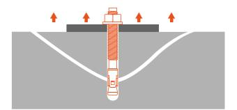
The size of the concrete failure cone will in most cases be three times the anchors effective embedment depth hef in diameter and therefore also has an influence on not only the spacing between any adjacent fixing but also the edge distance ac.
