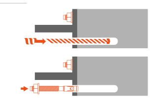
Flush fixings tends to work fine when a single fixing is being made and the item is not too heavy or large, that moving it may cause problems. However, a high degree of accuracy is required and unless done correctly may cause problems with multiple fixings.
